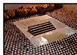
CDDOT Type D Inlet Parallel (20" Incline & Depressed)
