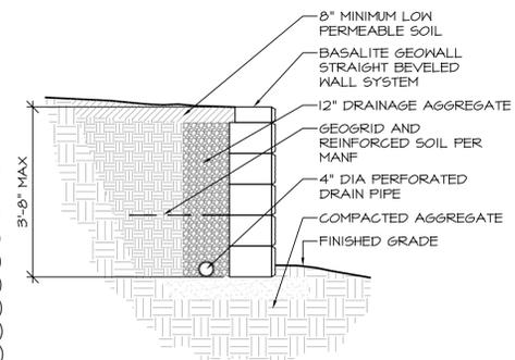
WALL SYSTEM TO BE INSTALLED PER MANUFACTURER'S RECOMMENDATIONS
