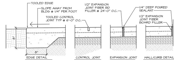
TYP CONSTRUCTION: 4" CONC SLAB W/ 6X6X10 GA WELDED WIRE FABRIC TYP ON 4" MIN BASE COURSE.
