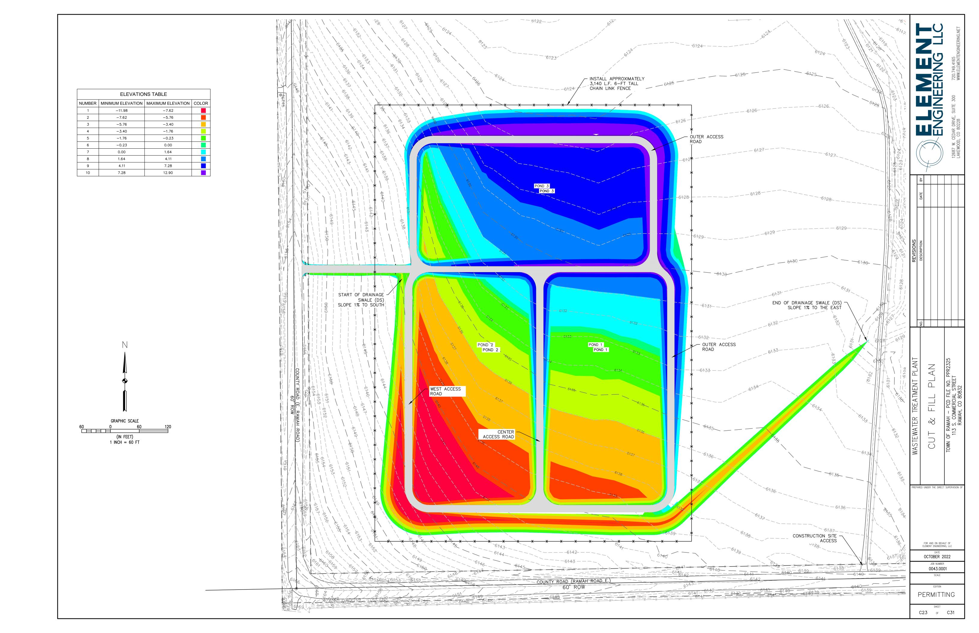
LINER MATERIAL: 45-MIL FPP-R (FLEXIBLE REINFORCED POLYPROPYLENE) OR 45-MIL LLDPE-R (LINEAR LOW
