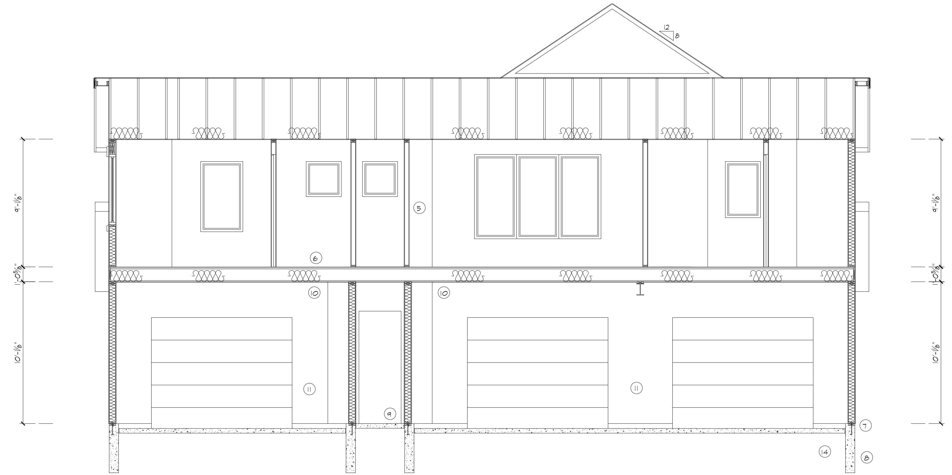
BUILDING SECTION 2 SCALE: 1/4"=1'-0" A-3
