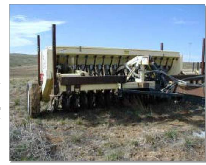
Photograph TS/PS-1. Equipment used to drill seed. Photo courtesy of Douglas County.
