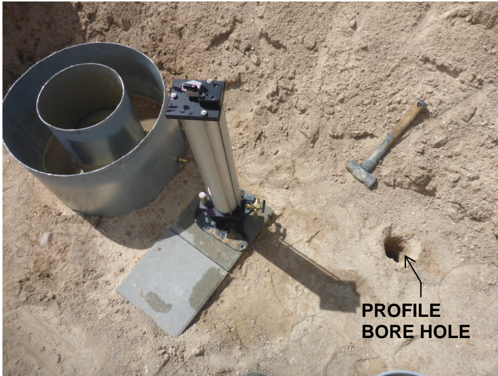
INFILTROMETER AND PROFILE BORE HOLE
