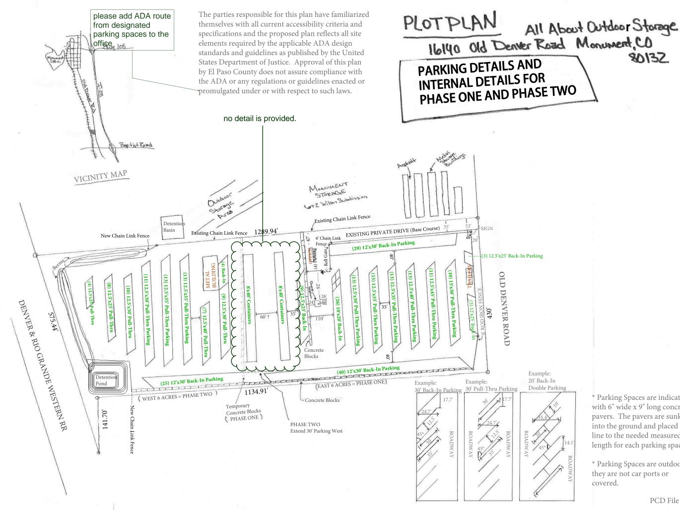
\* Parking Spaces are indicated with 6" wide x 9" long concrete pavers. The pavers are sunken into the ground and placed in a line to the needed measured length for each parking space.
