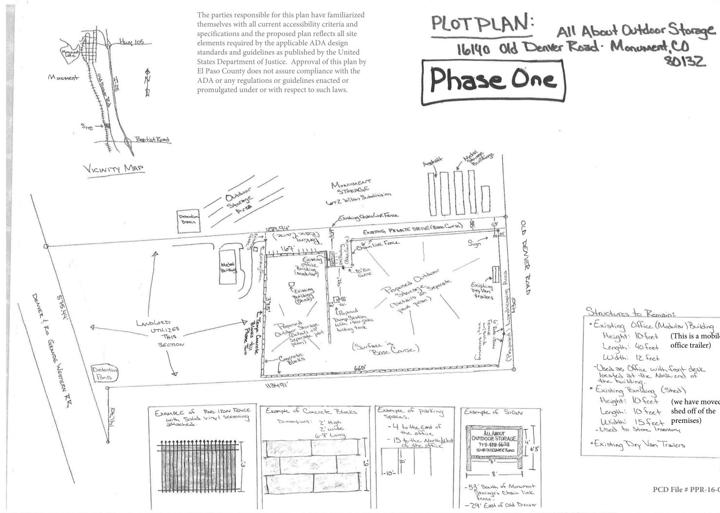
Structures to Remains · Existing Office (Modular) Building Height: 10 feet (This is a mobile Length: 40 Feet office trailer) Width: 12 feet -Osed as Office with front desk located at the North and of the building · Existing Pavilding (Shed) Height! 10 feet (we have moved this Length: 10 feet shed off of the Width: 15feet premises) - Used to Store Inventory · Existing Dry Van Trailers
