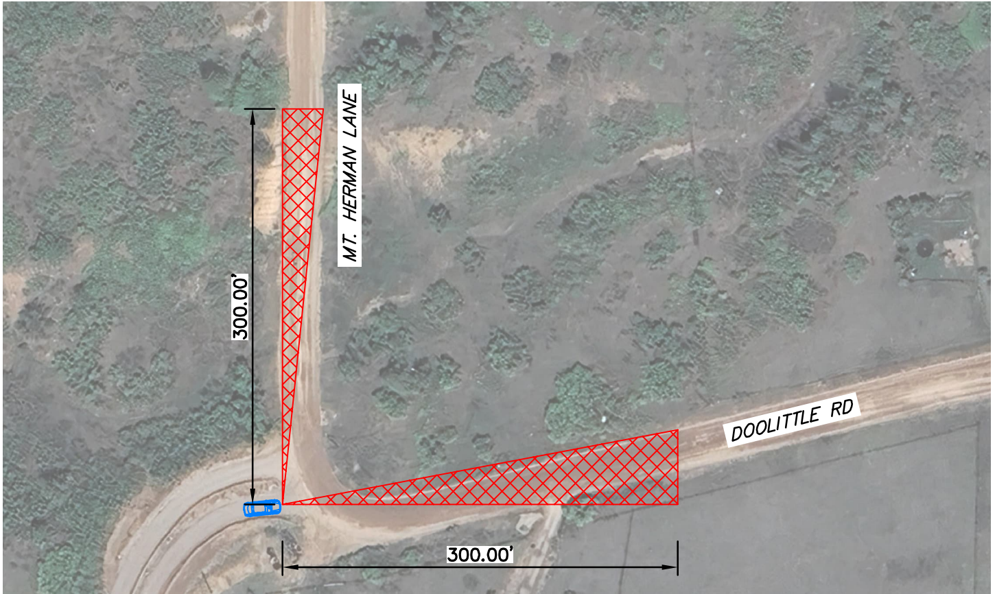
Figure 5 - Sight Distance Triangles
