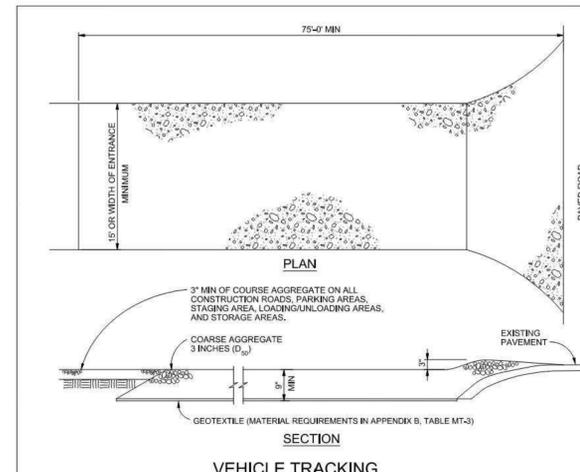
**VEHICLE TRACKING INSTALLATION REQUIREMENTS**
