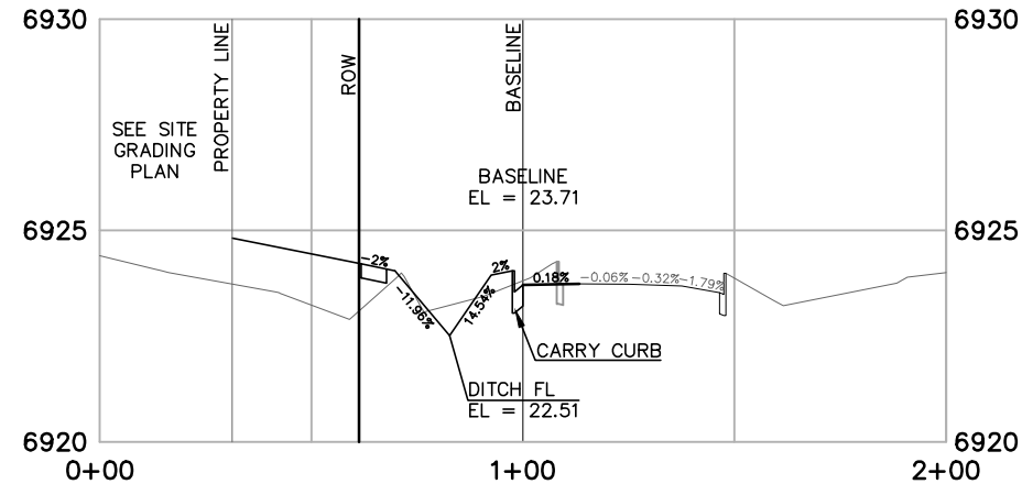
STAPLETON DRIVE SECTION 4+50.00 HORIZONTAL SCALE: 1" = 50' VERTICAL SCALE: 1"=5'
