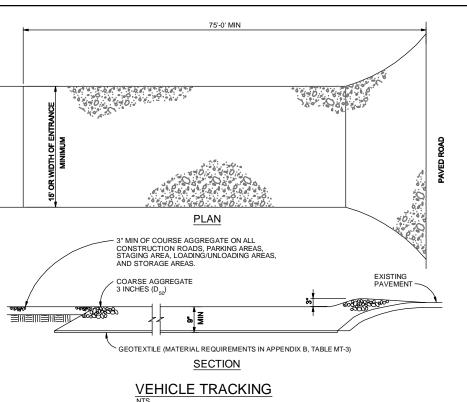
VEHICLE TRACKING NOTES INSTALLATION REQUIREMENTS . ALL ENTRANCES TO THE CONSTRUCTION SITE ARE O BE STABILIZED PRIOR TO CONSTRUCTION
