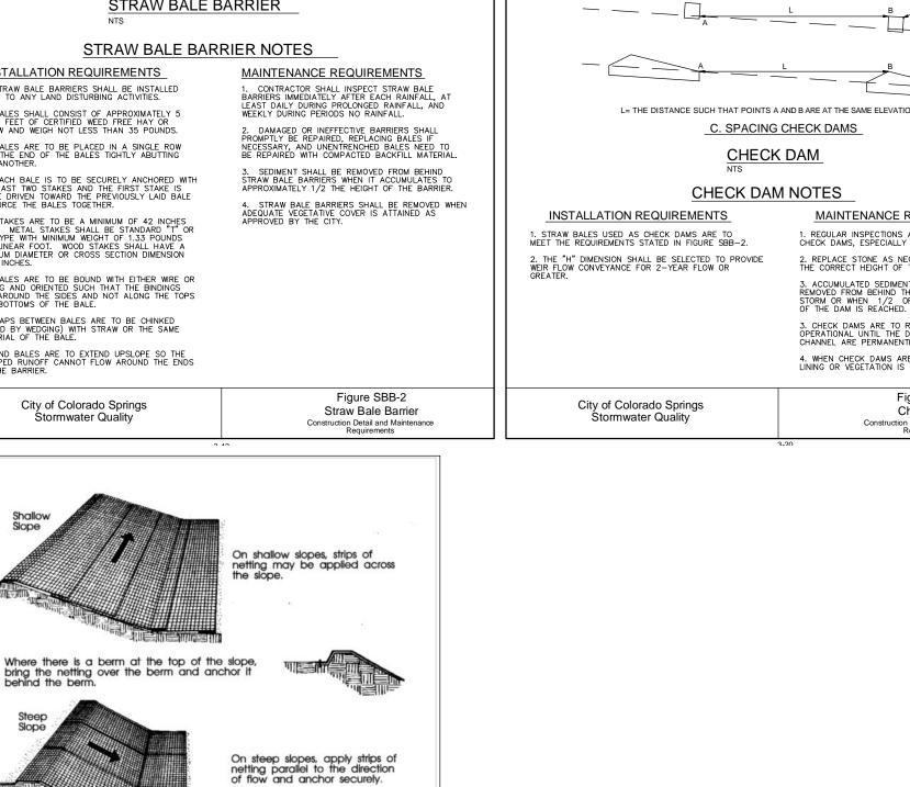
In ditches, apply netting parallel to the direction of flow. Use check slots every 15 feet. Do not join strips in the center of the ditch.
