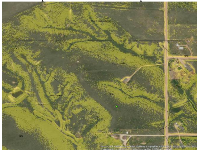
Figure 1. Slope map showing areas greater than 30% as calculated from a 1 meter digital elevation model (DEM) derived from LIDAR images.
