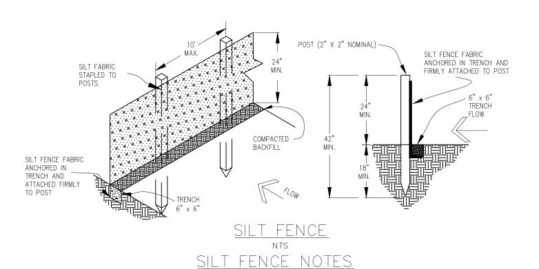
INSTALLATION REQUIREMENTS 1. SILT FENCES SHALL BE INSTALLED PRIOR TO ANY LAND DISTURBING ACTIVITIES.
