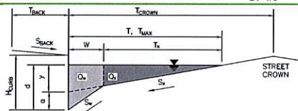
**Gutter Geometry (Enter data in the blue cells)**
