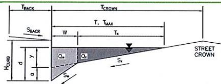
**Gutter Geometry (Enter data in the blue cells)**
