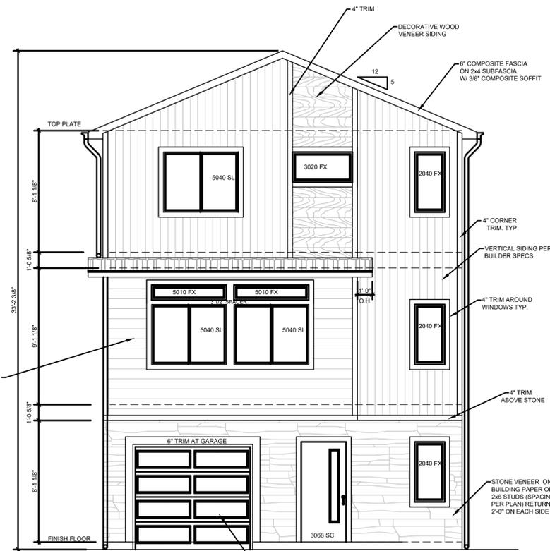
LAP SIDING ON BUILDING PAPER ON 7/16\" (MIN) PLYWOOD, O.S.B. OR STRUCTURAL WALL SHEATHING ON 2x6 WOOD STUDS (SPACING PER PLAN) W/ R-19 (MIN) BATT INSULATION
