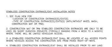
VTC-4. STABILIZED CONSTRUCTION ENTRANCE/EXIT
