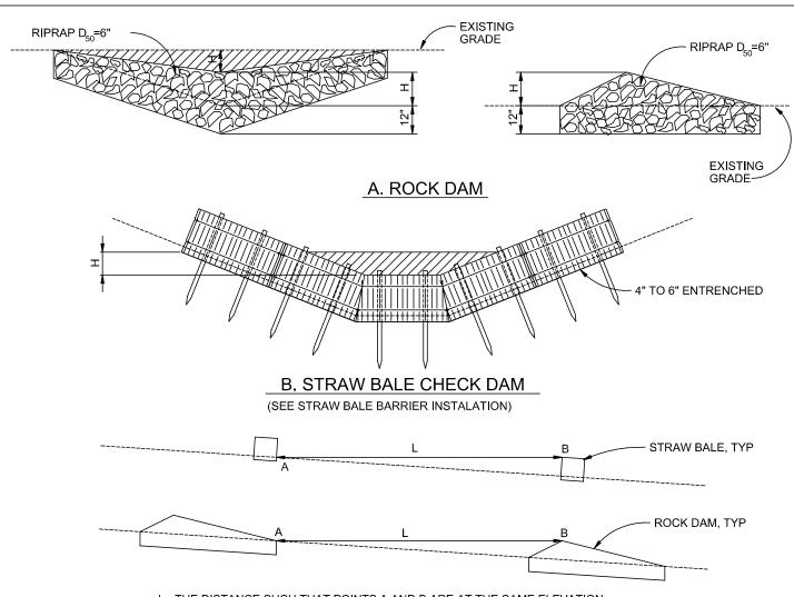
L= THE DISTANCE SUCH THAT POINTS A AND B ARE AT THE SAME ELEVATION.
