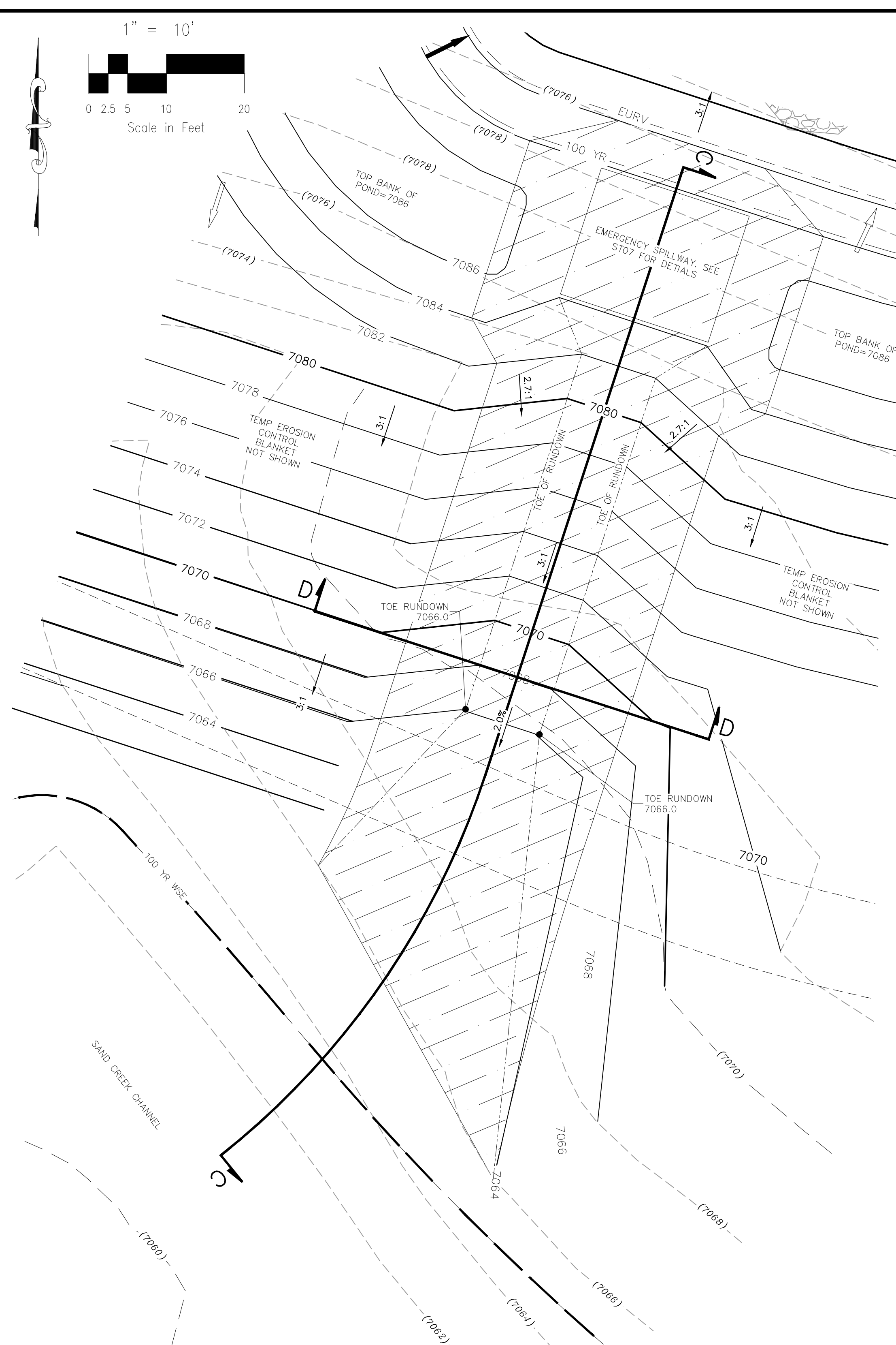
FDS POND 1 EMERGENCY SPILLWAY AND RUNDOWN TO SAND CREEK CHANNEL 1"=10'
