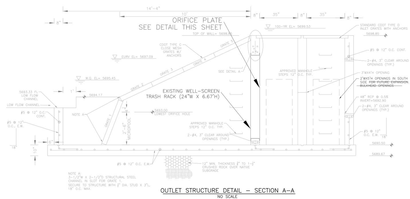
**OUTLET STRUCTURE DETAIL - SECTION A-A**
