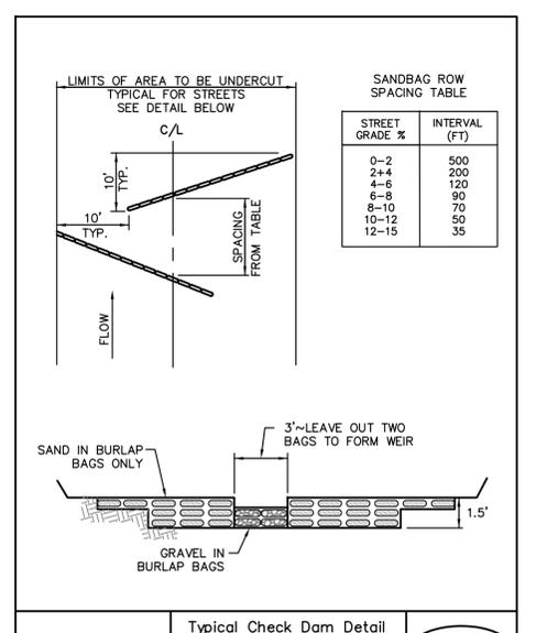
Typical Check Dam Detail Standard Drawing
