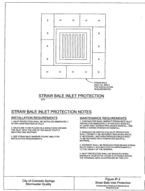
Figure IP-2 Straw Bale Inlet Protection Construction and Maintenance Requirements
