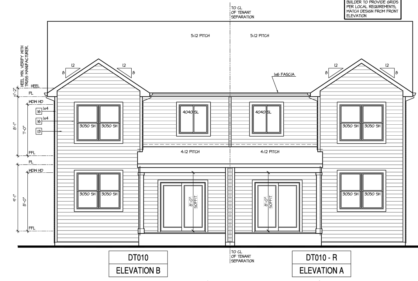
Rear Elevation - Building Type (DT010 + DT010) 'A-1/B-1' at Craw Space SCALE: 1/4"=1'-0" AT 22'50" LAYOUT, 1/8"=1'-0" AT 17'5" LAYOUT
