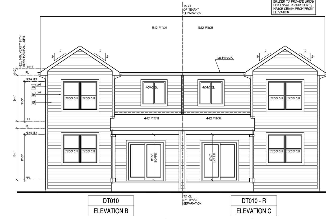
Rear Elevation - Building Type (DT010 + DT010) 'C-4/B-4' at Craw Space SCALE: 1/4"=1'-0" AT 22'50" LAYOUT, 1/8"=1'-0" AT 17'5" LAYOUT
