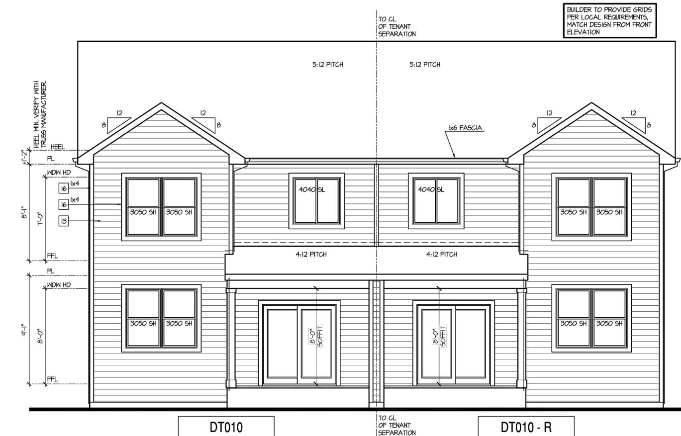
Rear Elevation - Building Type (DT010 + DT010) 'C'/'B' at Crawl Space
