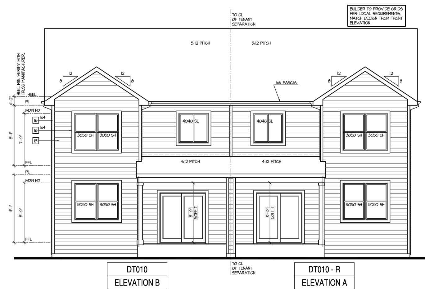
Rear Elevation - Building Type (DT010 + DT010) 'A'/'B' at Crawl Space
