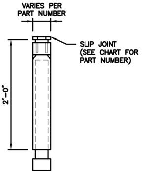
NOTE: CONTRACTOR TO INSTALL EXPANSION FITTING SLIP JOINT AT METER CENTER CONDUIT TERMINATION, AS PER LOCAL UTILITY POLICY, ORDINANCE AND/OR SPECIFIED REQUIREMENT.
