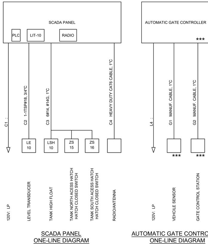
**SCADA PANEL ONE-LINE DIAGRAM**
