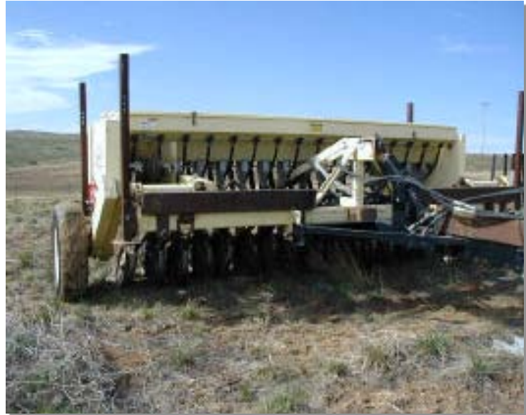
Photograph TS/PS -1. Equipment used to drill seed. Photo courtesy of Douglas County.
