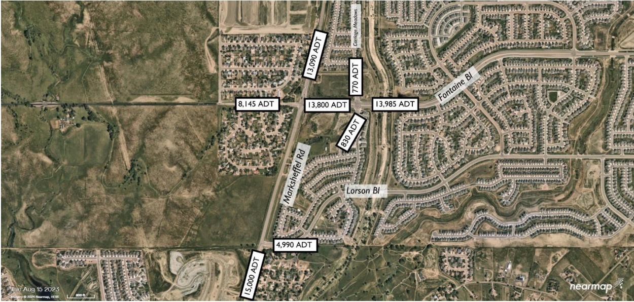
Figure 5. Existing Conditions Daily Traffic Volumes
