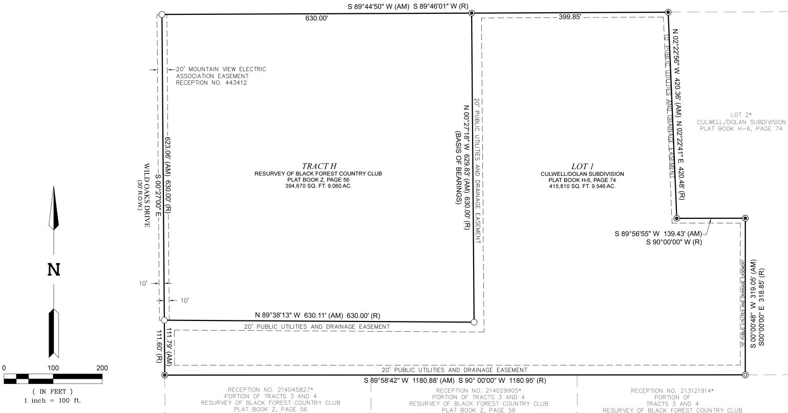
AS PLATTED SET 5/8"X18" REBAR WITH ORANGE PLASTIC CAP "PLS 30106" FOUND 1/2" REBAR WITH PLASTIC CAP ILLEGIBLE
