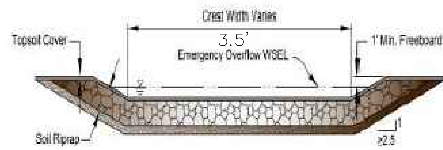
Figure 13-12c. Emergency Spillway Protection
