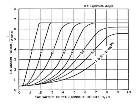
Figure 9-36. Expansion factor for rectangular conduits
