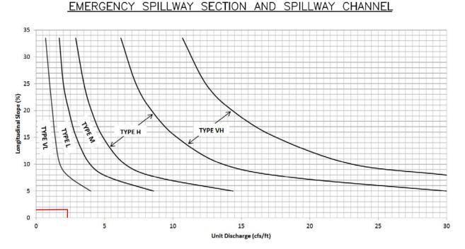
Figure 12-21. Embankment protection details and rock sizing chart (adapted from Arapahoe County)
