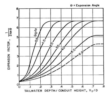
Figure 9-35. Expansion factor for circular conduits
