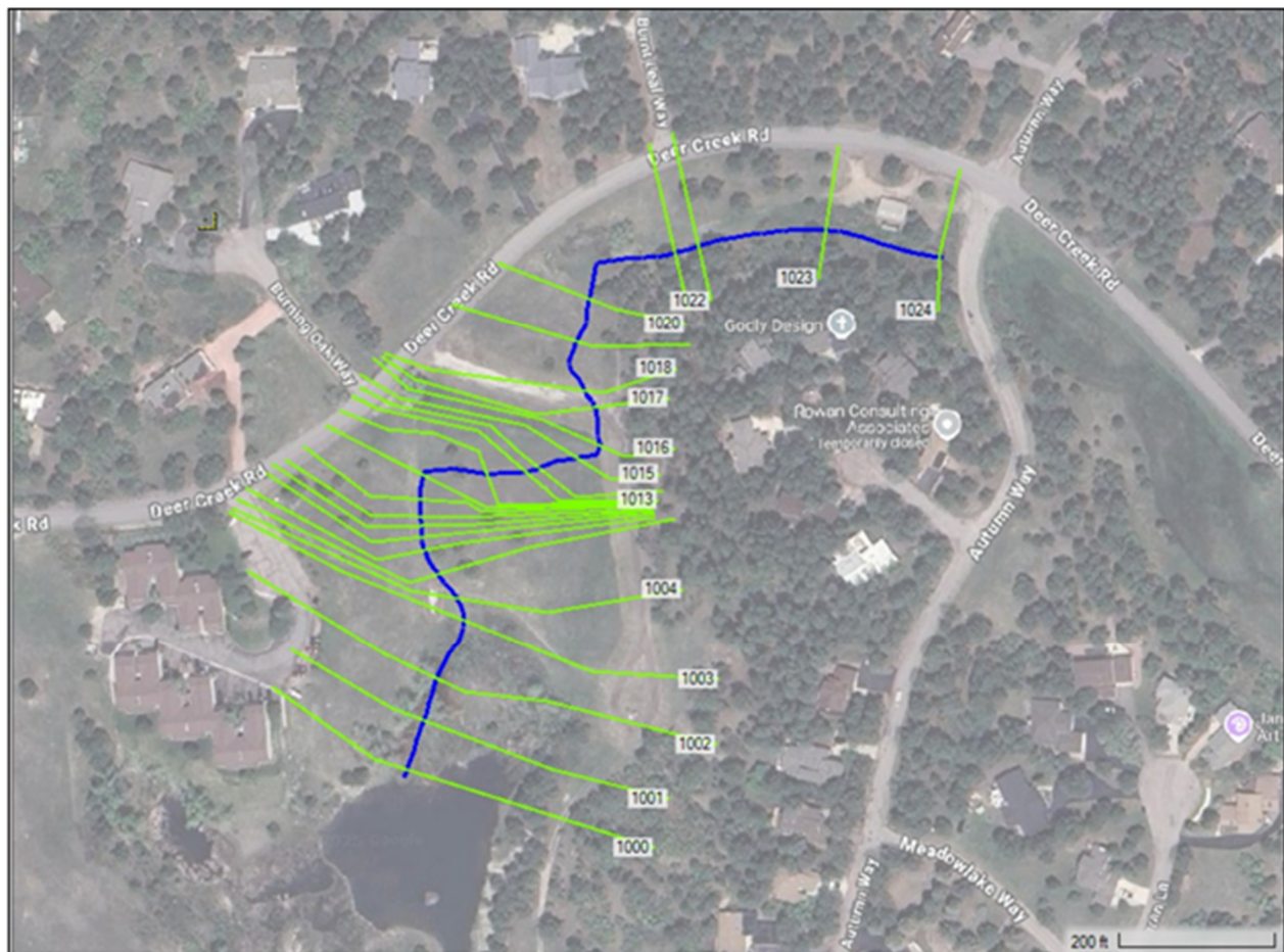
Figure 3. Pre-project Model Cross-sections
