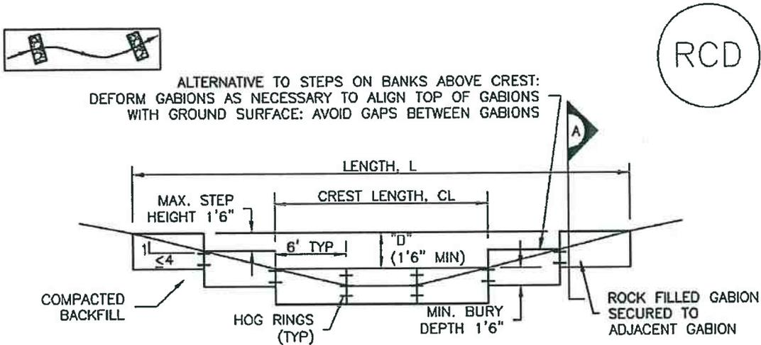
REINFORCED CHECK DAM ELEVATION VIEW
