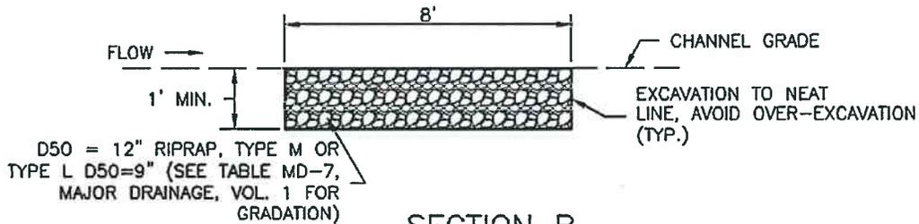
D50 = 12" RIPRAP, TYPE M OR TYPE L D50=9" (SEE TABLE MD-7, MAJOR DRAINAGE, VOL. 1 FOR GRADATION)
