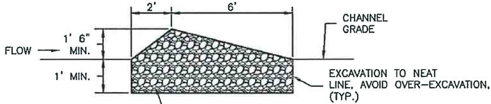
D50 = 12" RIPRAP, TYPE M OR TYPE L D50= 9" (SEE TABLE MD-7, MAJOR DRAINAGE, VOL. 1 FOR GRADATION)
