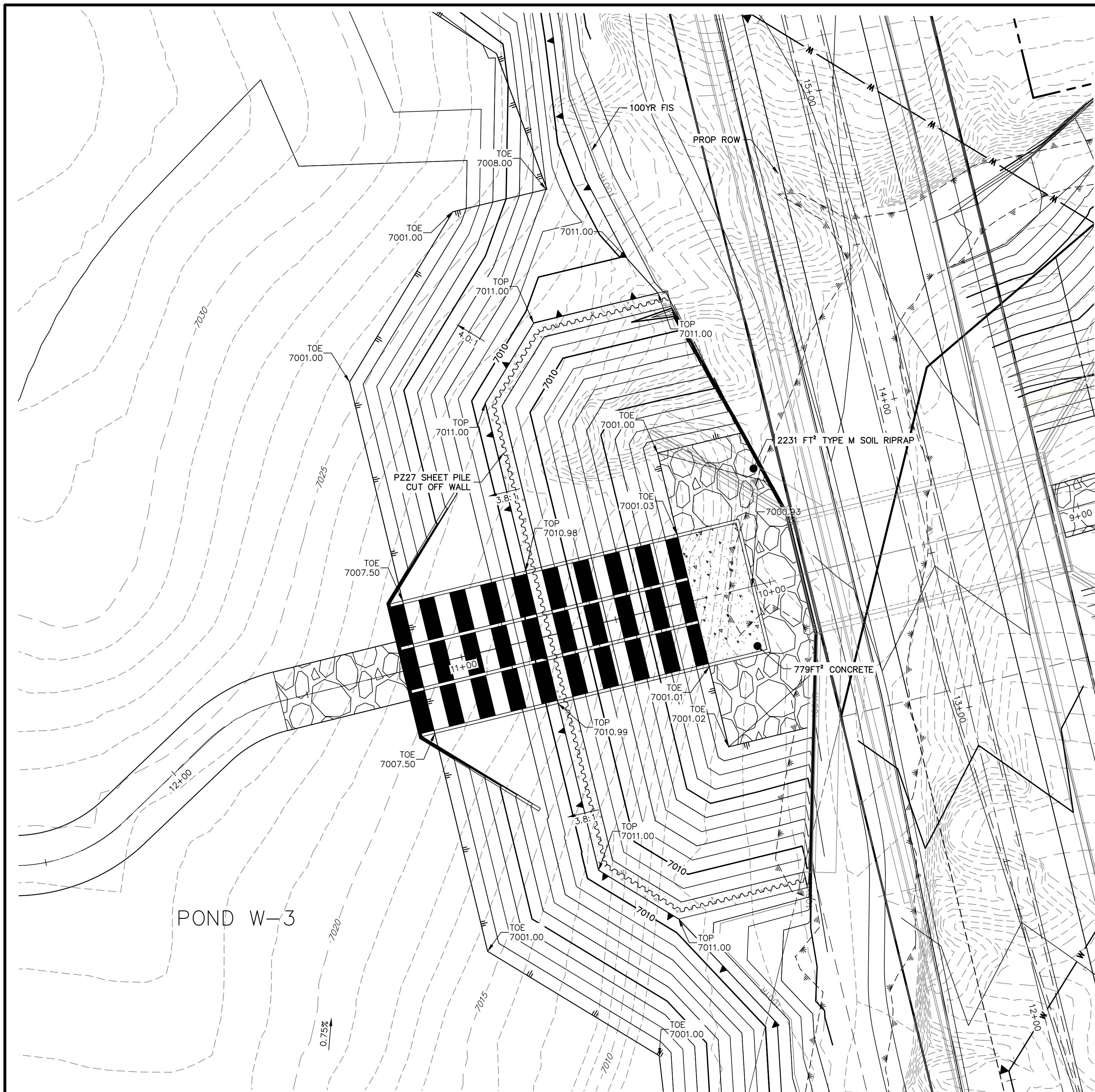
POND W-3 OVERFLOW WEIR SCALE: 1"=20'
