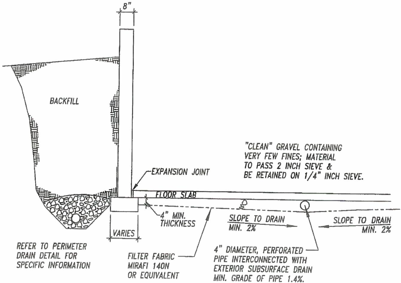
4.11c Detail Room/Drawings/Underlab Capillary Break Drain Area/Issued/6/12/2007 12:11:56 PM 1/4"
