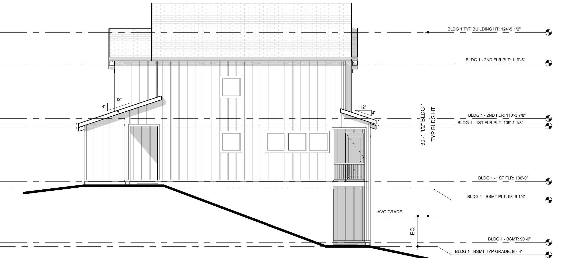
1 RIGHT ELEVATION - BUILDING TYPE 1 1/8" = 1'-0"
