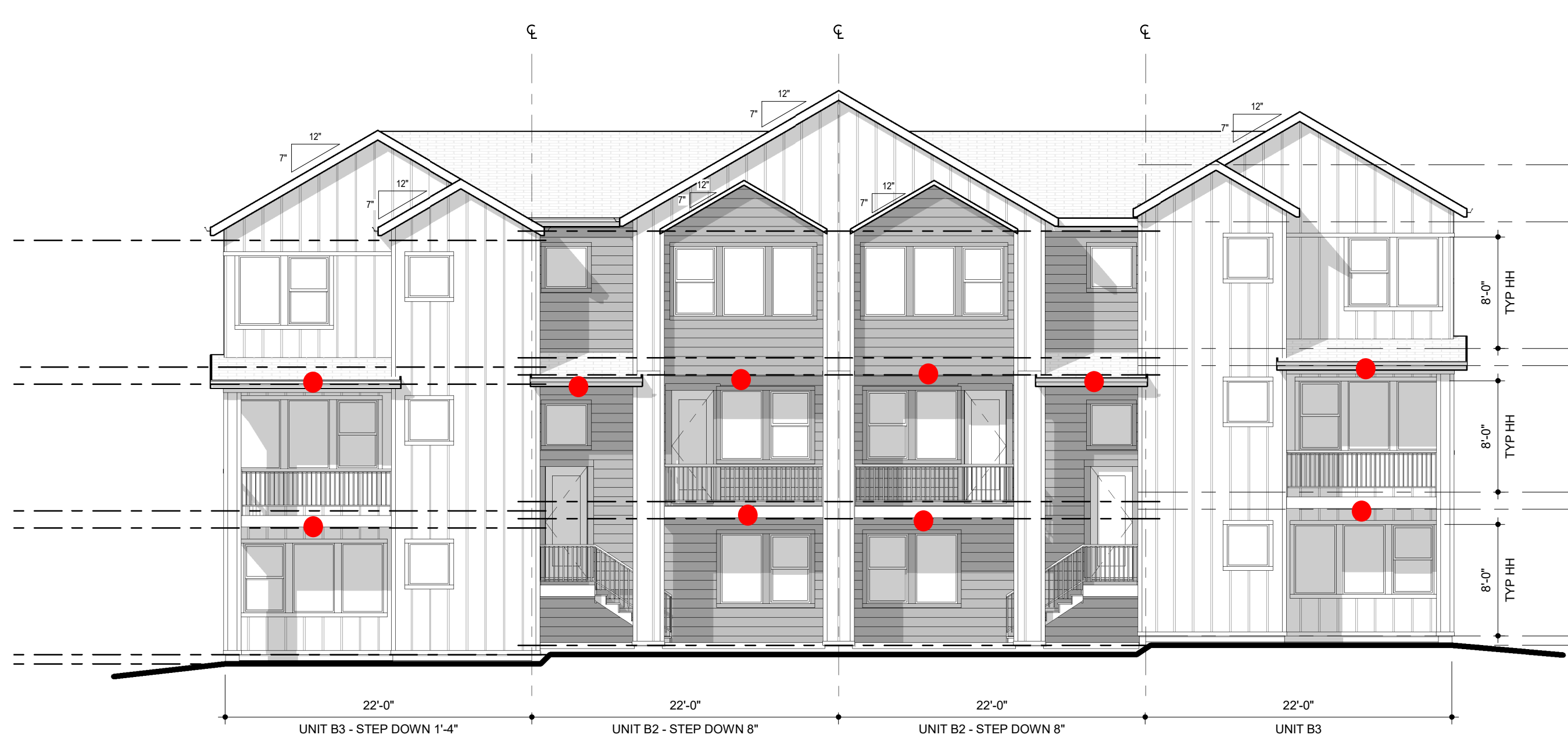
2 FRONT ELEVATION - BUILDING TYPE 2 1/8" = 1'-0"
