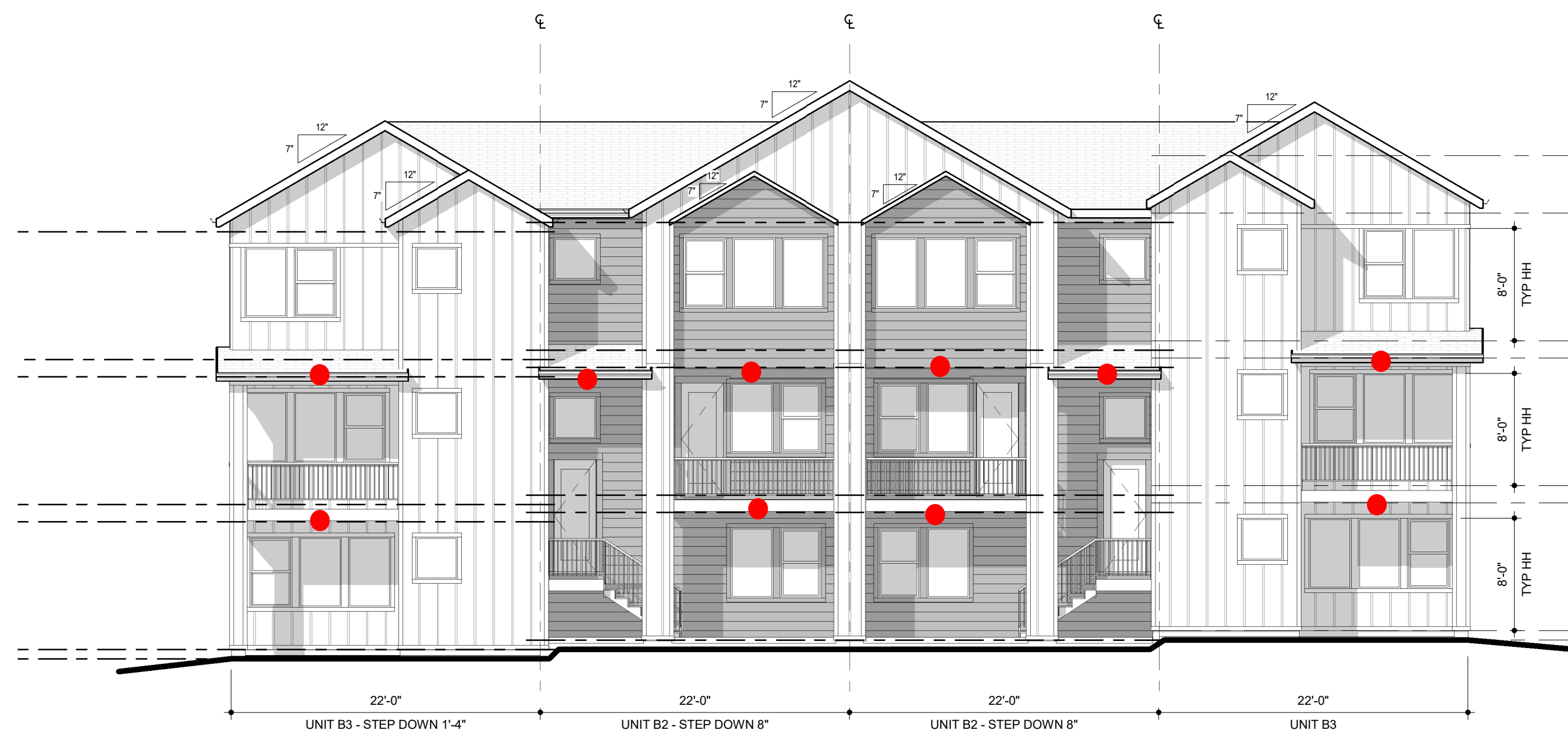
2 FRONT ELEVATION - BUILDING TYPE 2 1/8" = 1'-0"
