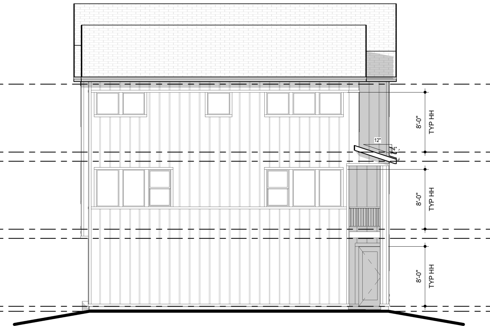
3 LEFT ELEVATION - BUILDING TYPE 2 1/8" = 1'-0"
