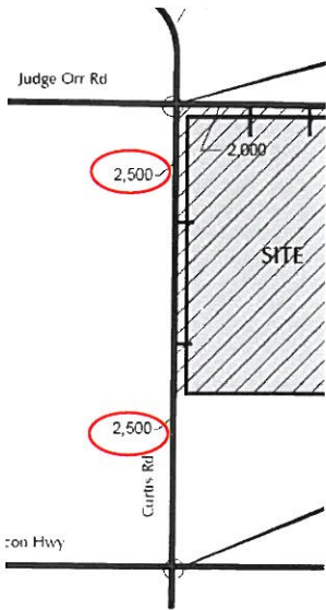
Existing ADTs on Curtis Road
