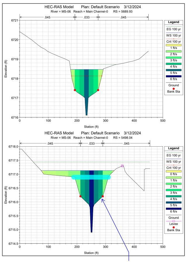
Consider adding a cutoff wall at the full graded width or at least to edges of 3 fps limits
