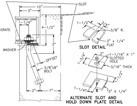
**OVERFLOW GRATE INSTALLATION DETAIL**
