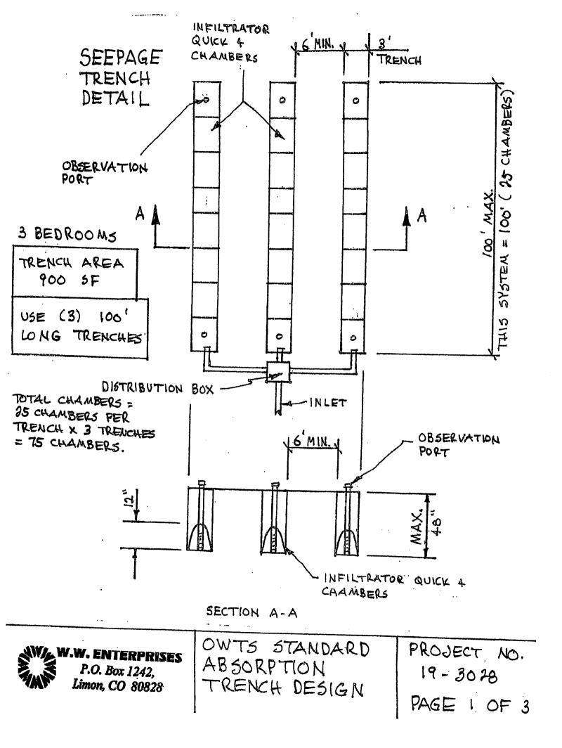
KEY A 1000 GAL. 2 COMP. SEPTIC TANK FOR 3 BEDROOMS B 4" SCHED. 40 PVC PIPE FROM SEPTIC TANK TO D-BOX. C DISTRIBUTION BOX ELEV. MAX 3.5' DEPTH D 4" SCHED. 40 PVC DISCHARGE PIPES -D-BOX TO TRENCHES E OUTLET PIPE FLOWLINE PER TANK. BASEMENT SLAB PER GRADE. F SEPTIC TANK OUTLET ELEV. = MAX. 4' DEPTH G TRENCHES - BOTTOM MAX. 4' BELOW GRADE
