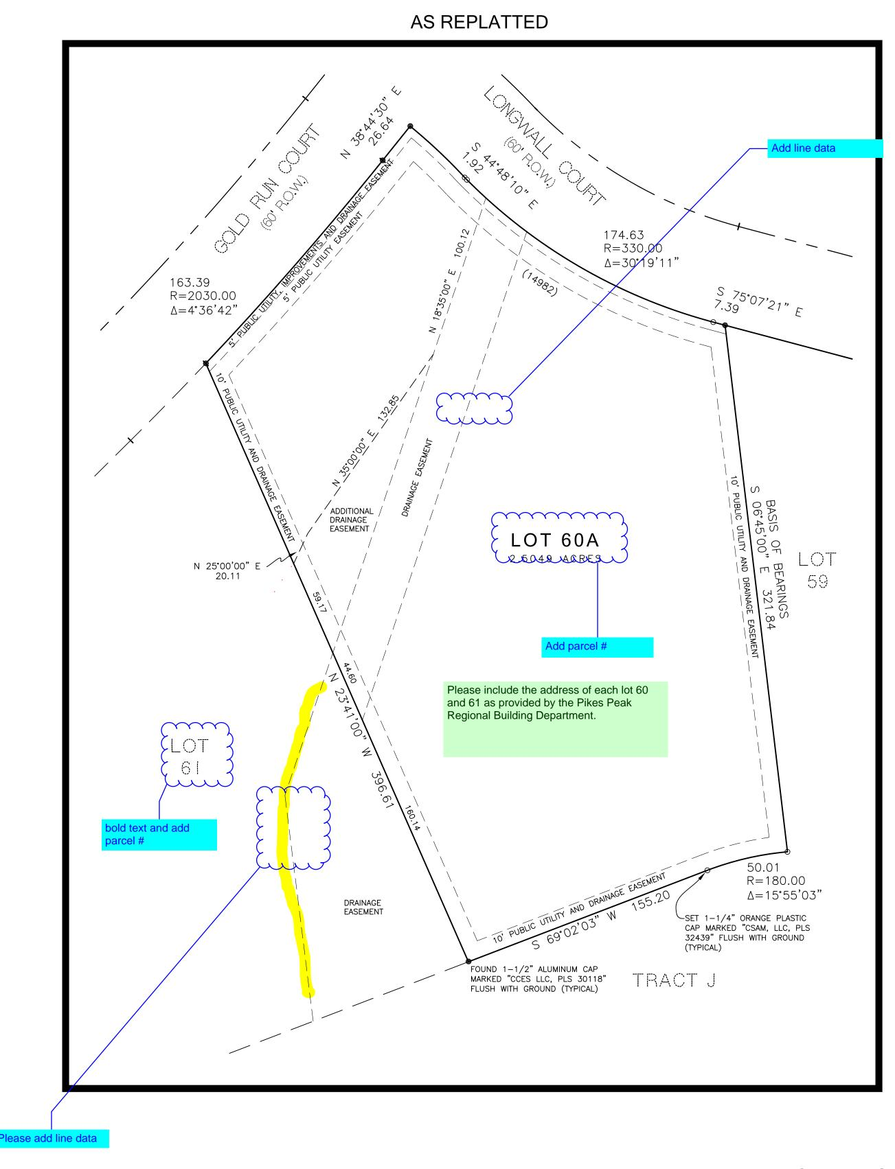
Suggest showing both lots 60 and 61 with drainage easement on both lots or recording change by separate instrument only.
