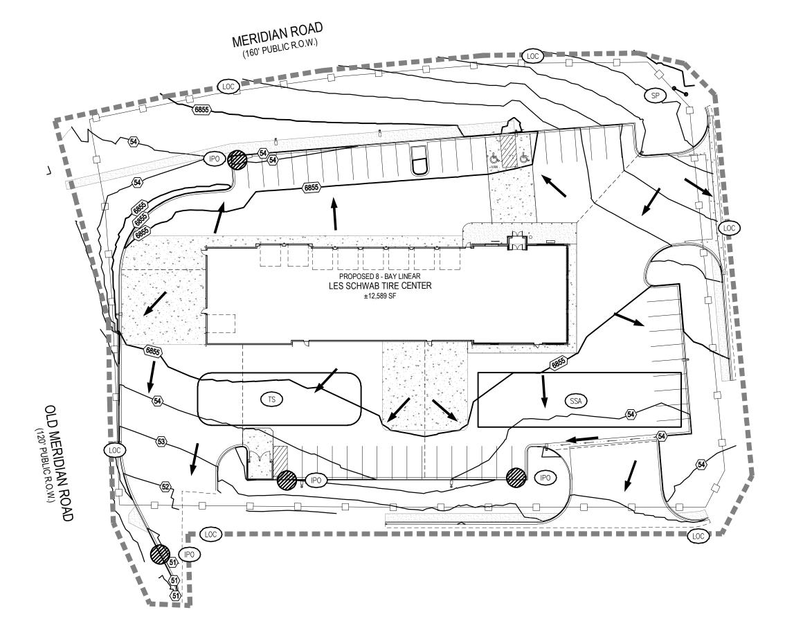
POST-PAVING STORM WATER MANAGEMENT PLAN SCALE: 1"=40
