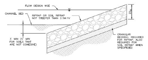
THICKNESS - 2\*D50 = 24" SIDE SLOPE - 2.5:1 BURY DEPTH - 5' (ASSUME NOT COHESIVE)
