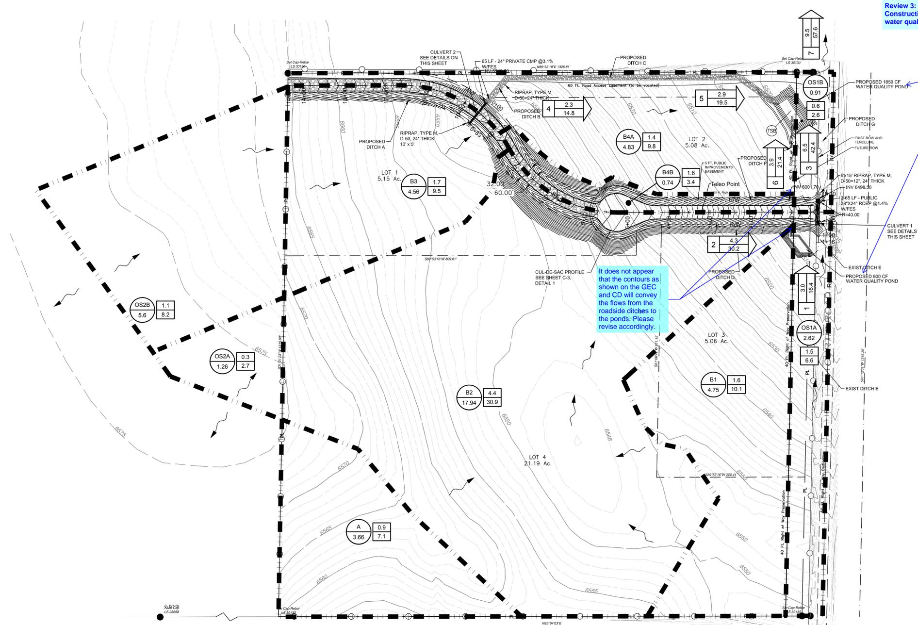
It does not appear that the contours as shown on the GEC and CD will convey the flows from the roadside ditches to the ponds. Please revise accordingly.
