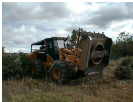
Figure 3. Mechanical treatment using a Hydroaxe®.
