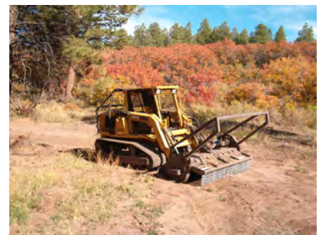
Figure 4. Mechanical treatment using a timberaxe.
