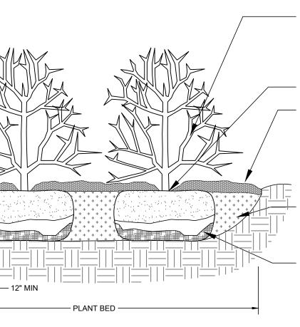
SET SHRUBS VERTICAL. SHRUB SPACING AS PER PLANS. LAYOUT VARIES. FINISHED GRADE OF SHRUB BED TO BE 2" BELOW ADJACENT FINISH GRADE AT EDGE TO HOLD MULCH.
