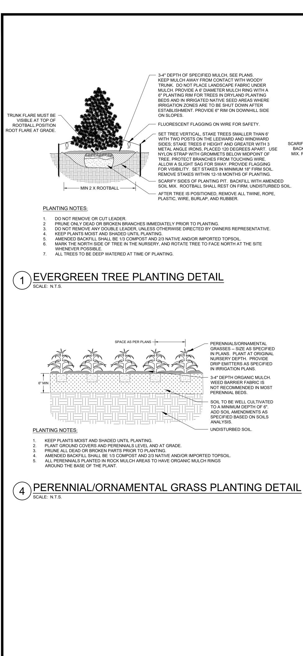
SCARIFY SIDES OF PLANTING PIT. BACKFILL WITH AMENDED SOIL MIX. ROOTBALL SHALL REST ON FIRM, UNDISTURBED SOIL.
