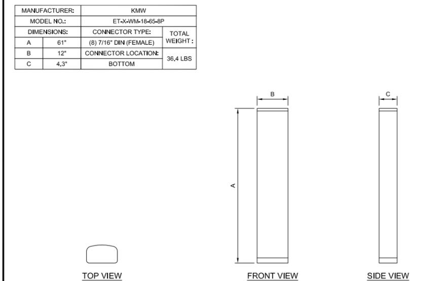
**(N) AND (E) RRUS MOUNTING DETAIL** 24"x36" SCALE: NTS 11"x17" SCALE: NTS **5**
