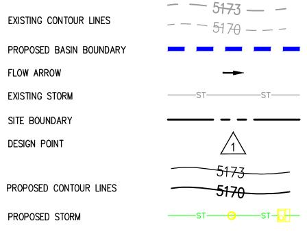
5-YR RATIONAL BASIN DESIGNATION OS 1 C COEFFICIENT AREA C MINOR 1.23 0.45 AC 0.67 BASIN SIZE \_\_\_\_ IN ACRES 100-YR RATIONAL C COEFFICIENT BASIN DESIGN POINT
