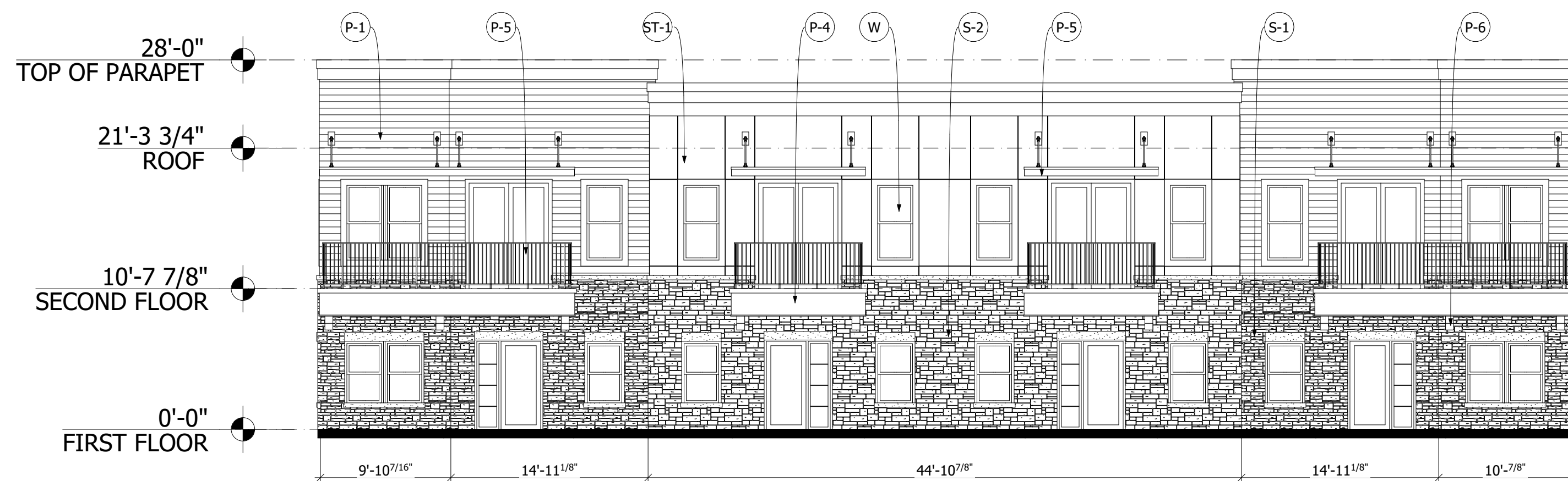
1 TOWNHOUSE 4, 6, 8, & 9 - SOUTH ELEVATION GLA_23 SCALE: 1/8" = 1'-0"
