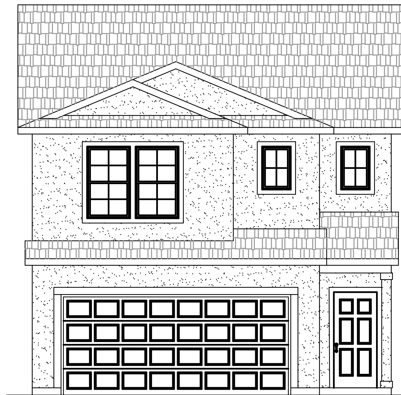
FRONT ELEVATION-TRADITIONAL - STUCCO 1/4"=1'-0"
