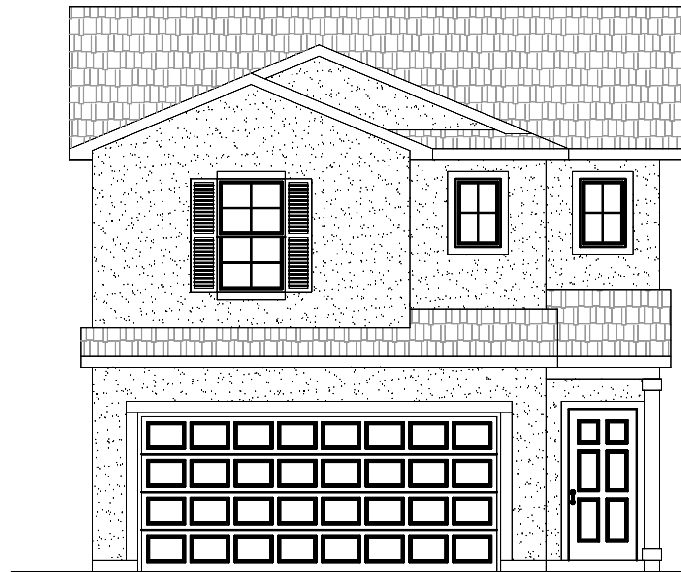
FRONT ELEVATION-TRADITIONAL - STUCCO 1/4"=1'-0"
