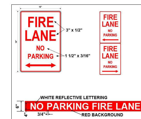
1 FIRE LANE/NO PARKING SIGN DETAIL NTS
